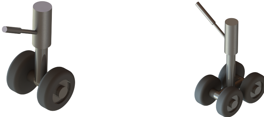
(a) Nose landing gear uses a two-wheel bogie to support the weight of the front of the aircraft
